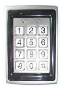
5399 is a standalone access control system, stainless steel case for vandal proof, 500 users and 500 passwords, adopting 125 KHz proximity card and programmed on keypad with no software needed, so it doesn't provide audit trial record. It also possesses alarm functions, and includes 4 access methods: password, password + card, password + password, card + card.
